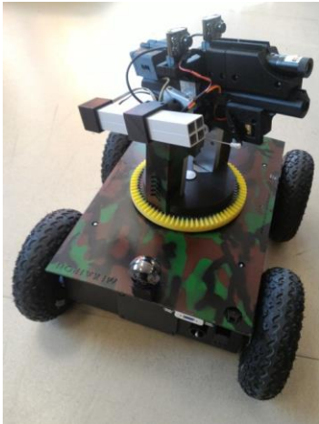
Figure 7. Real-time remote-controlled mobile robot platform
