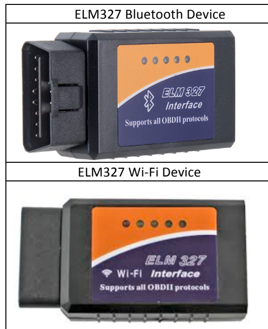
Figure 1. Wireless ELM327 Devices
