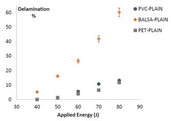
Figure 3. Comparison of the damaged area of the PVC–plain, PET–plain and balsa wood–plain cored sandwich composite structures
