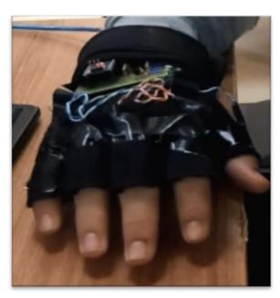
Figure 2. First version haptic glove
