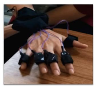
Figure 3. Second version haptic glove
